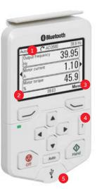
With the customizable Home views you can monitor the values that matter most, e.g. pump speed, water flow or pressure, torque or motor temperature. Select the signals from a ready-made list or choose user defined parameters.
