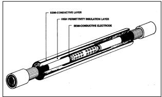
All finished bodies are tested after manufacture and undergo AC Withstand and Partial Discharge testing.
