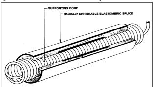
QS1000 is injection moulded and consists of three layers. A semi-conductive electrode which forms a Faraday Cage around the connector, a high permittivity insulation layer which both insulates and stress controls, and an outer semi-conductive layer which ensures all screens are at earth potential.
